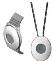
Your personal help button has an open air range of 300m+ to EVA. It regularly checks its battery and tests with EVA to ensure it is in contact. Tests are automatic and any issues are reported to your Alarm Receiving Centre (ARC).
